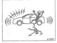
The theft deterrent system is designed to deter vehicle theft. This system flashes turn signal lights and sounds the alarm if someone attempts to damage or break into your vehicle. Furthermore, when the interior light switch is in the "DOOR" position, the interior light turns on.
