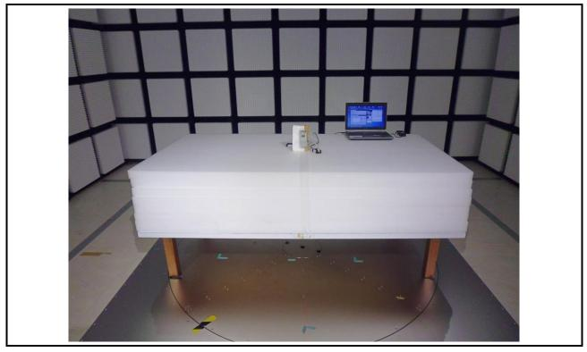
**Radiated Emission Below 1GHz Test**
