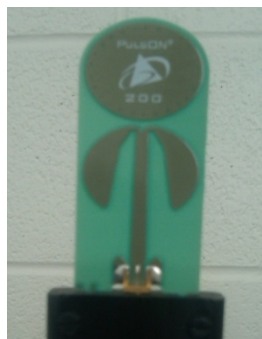
Figure 39. Pulse ON 200 UWB antenna features a microstrip-to-dual-notch transition.
