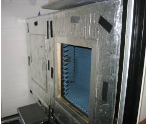
Figure 23. The anechoic chamber (left) used for testing antennas eliminating secondary reflections, and the interior of the anechoic chamber (right) containing the horn antenna on the left and the tested antenna on the right
