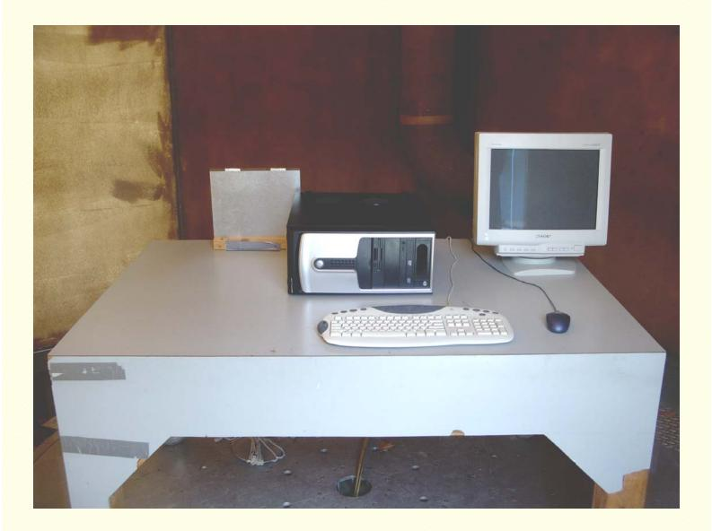
Radiated Emissions Measurement (Front View) Setup
