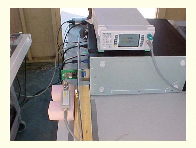
Maximum Peak Output Power Measurement Setup
