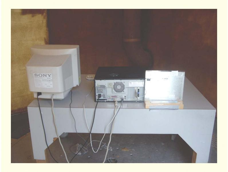
Radiated Emissions Measurement (Rear View) Setup
