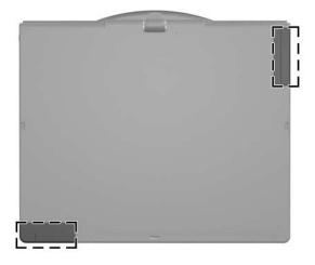
For optimal transmission, keep the areas immediately around the antennae free from obstructions.
