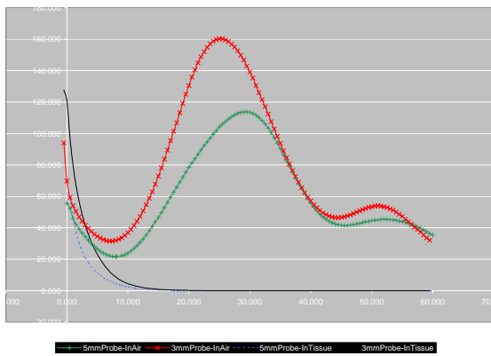
Figure 5: Comparison between the 2.8mm and 4.9mm probes in air and liquid-tissue with the WR159 waveguide.
