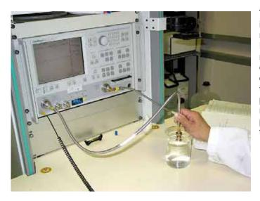
Tissue used during the SAR assessment calibrated prior to use in the measurement process. **APREL** Laboratories use the co-axial probe method for all tissue calibration exercises. Tissue which is being used over a period of 24 hours is re-calibrated to ensure that no change to the dielectric affect properties will the SAR measurement process. The table below provides details of the results from the tissue equivalent dielectric calibration.
