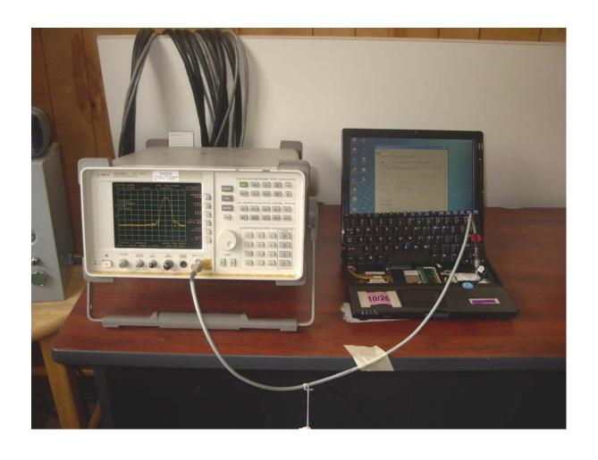
Conducted Emissions at Antenna Terminal Setup
