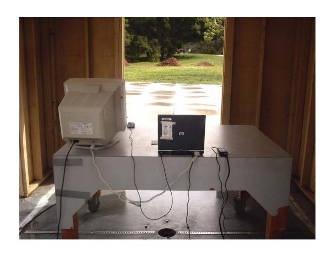
Radiated Emissions Measurement (Rear View) Setup
