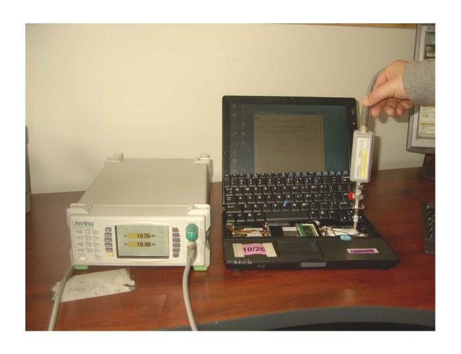
Maximum Peak Output Power Measurement Setup
