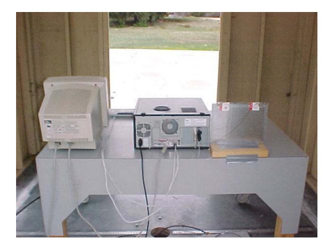
Radiated Emissions Measurement (Rear View) HP Altima Antenna Setup
