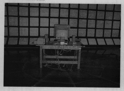
Radiated emission back connection details
