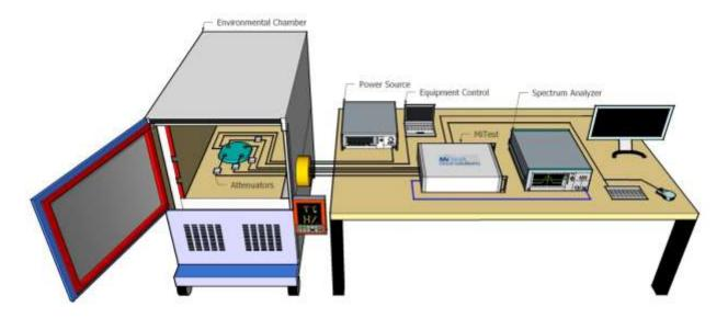
A full system calibration was performed on the test station and any resulting system losses (or gains) were
