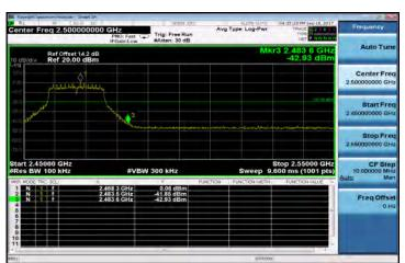
802.11n\_HT20: Band Edges Test Data CH-High
