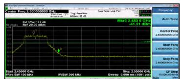
802.11g: Band Edges Test Data CH-12
