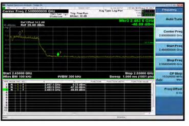
802.11n\_HT40: Band Edges Test Data CH-10
