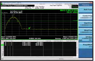
802.11b: Band Edges Test Data CH-12
