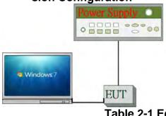
Fig. 2-3 Conducted (AC powerline) **Emission Configuration**
