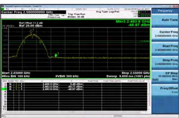
802.11b: Band Edges Test Data CH-13
