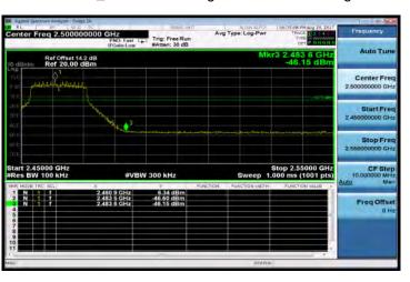
802.11n\_HT20: Band Edges Test Data CH-13
