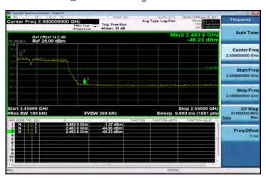
802.11n\_HT40: Band Edges Test Data CH-11
