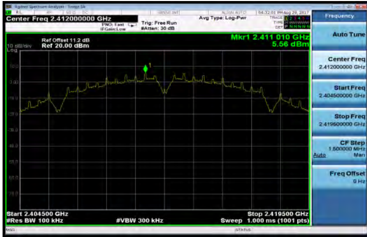
802.11b PSD for Bandedge Limit(CH-High)
