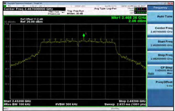
802.11g PSD for Bandedge Limit(CH-13)
