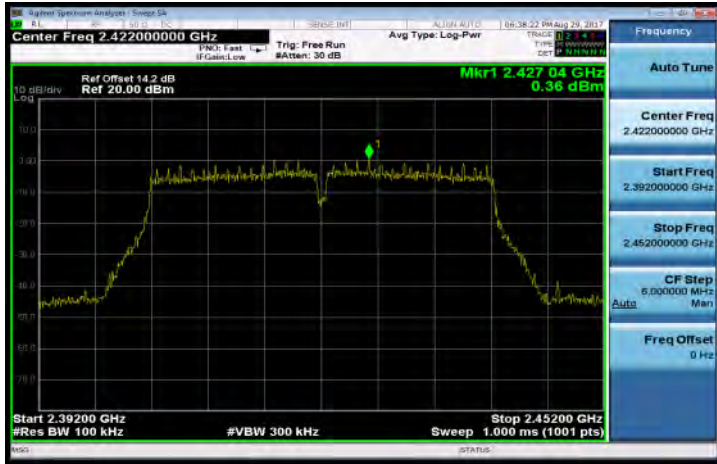
802.11n_HT40 PSD for Bandedge Limit(CH-High)
