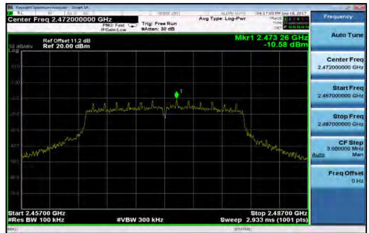
802.11g PSD for Bandedge Limit(CH-13)
