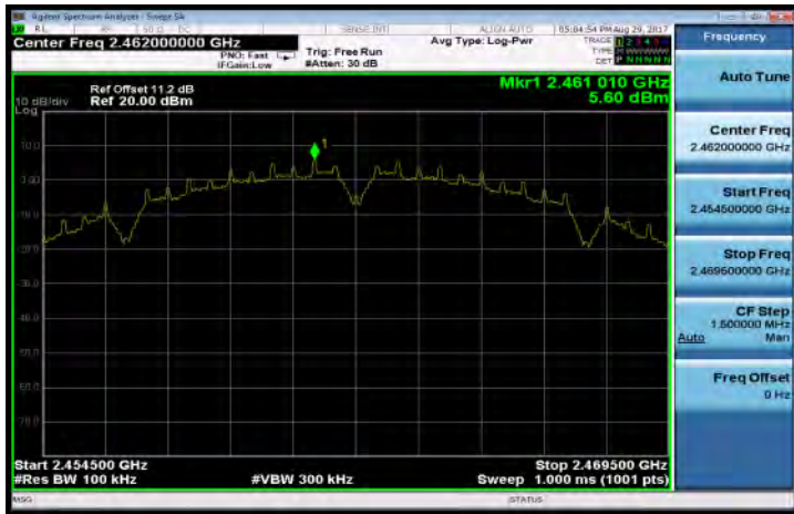
802.11b PSD for Bandedge Limit(CH-High)
