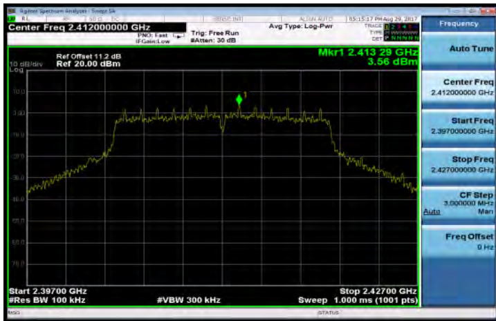
802.11g PSD for Bandedge Limit(CH-High)
