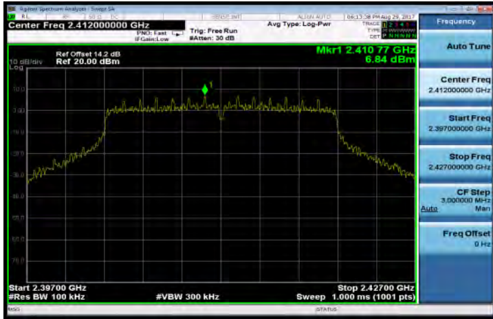
802.11n_HT20 PSD for Bandedge Limit(CH-High)
