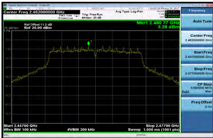
802.11g PSD for Bandedge Limit(CH-High)
