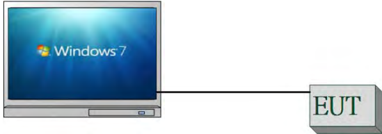
Fig. 2-1 Conducted (Antenna Port) Emission Configuration
