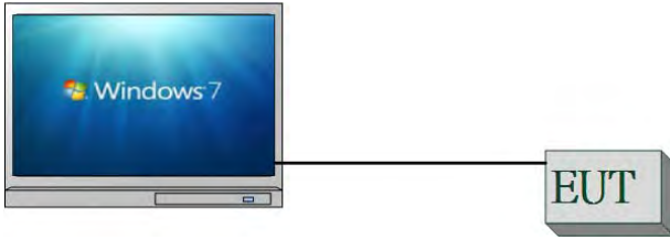
Fig. 2-2 Conducted (Antenna Port) Emission Configuration
