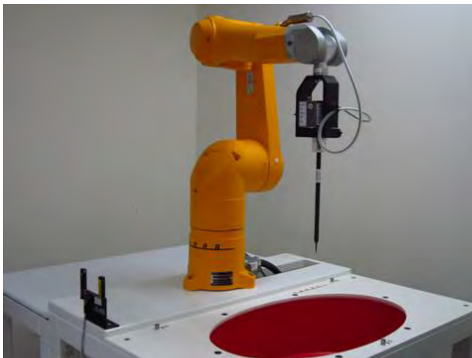
Fig.1 Photograph of the SAR measurement system
