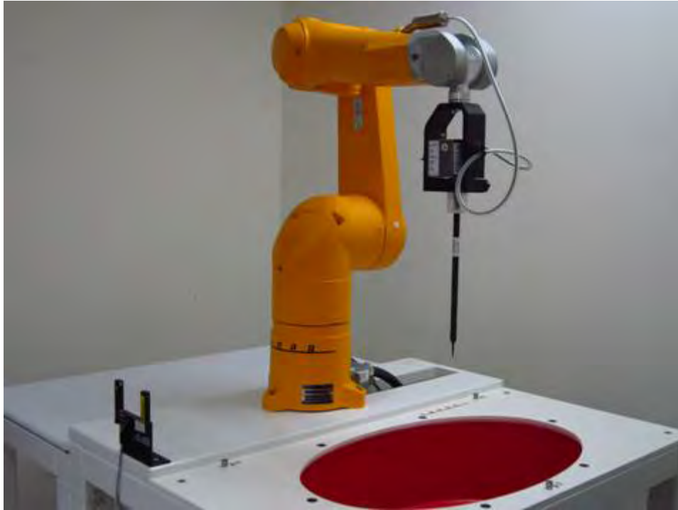
Fig.1 Photograph of the SAR measurement system
