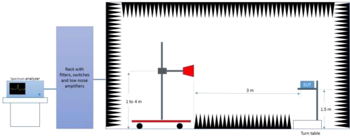
*Radiated Setup 6.4 GHz - 18 GHz*
