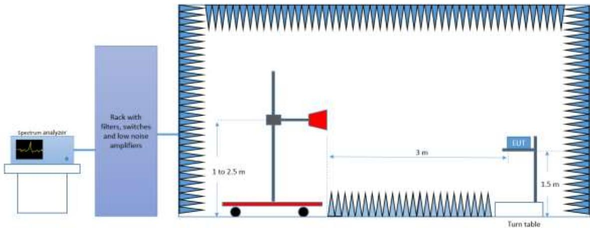
*Radiated Setup 18 GHz – 26.5 GHz*
