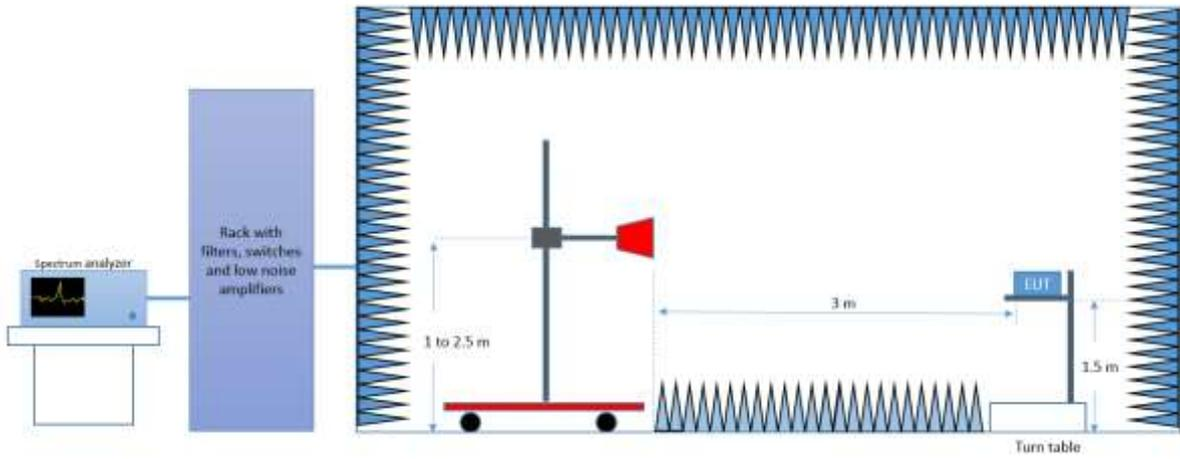
*Radiated Setup 18 GHz – 26.5 GHz*
