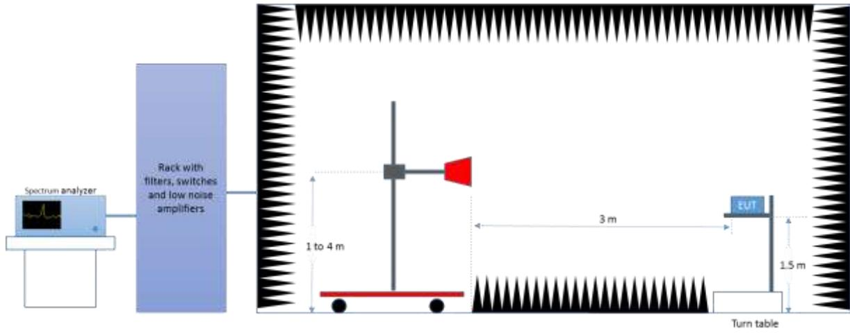
*Radiated Setup 6.4 GHz – 18 GHz*
