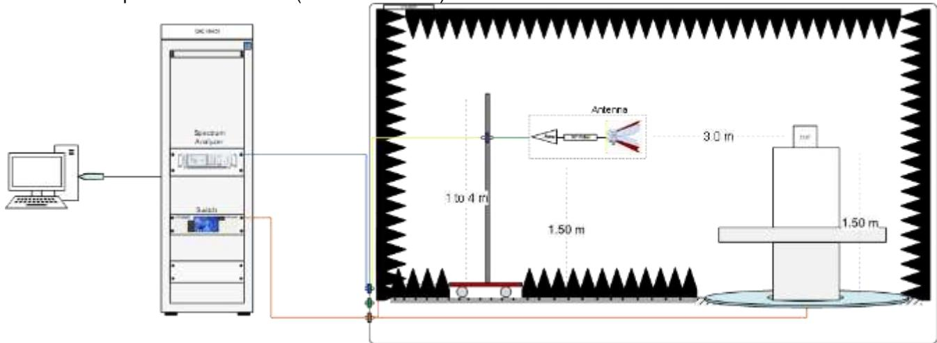
**Radiated Setup 18 GHz – 40 GHz (Transmitter tests)**
