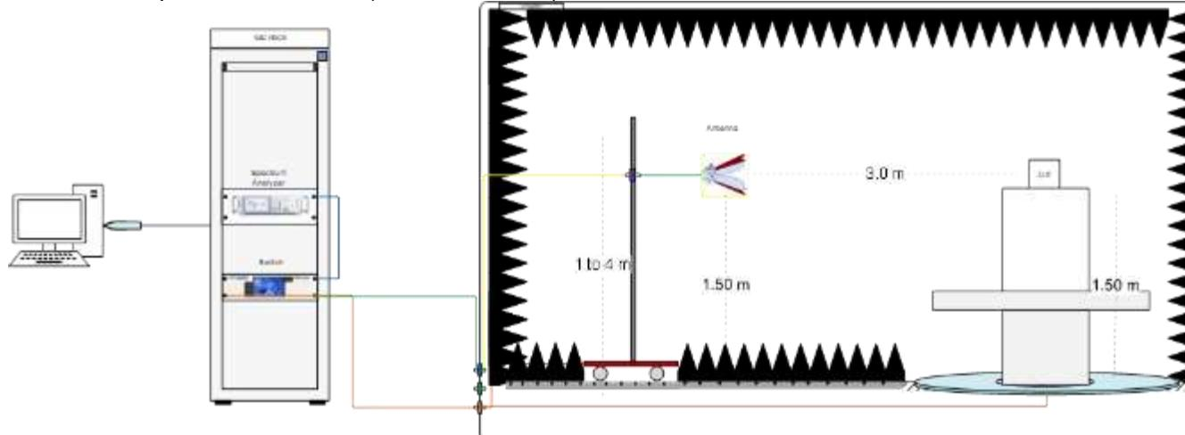
**Radiated Setup 6.4 GHz – 18 GHz (Transmitter tests)**
