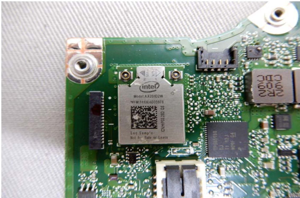
WLAN / BT Module-1 (Model No.: AX201D2W)
