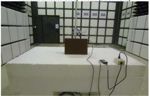
Radiated Emission Set up Photos (Above 1GHz)
