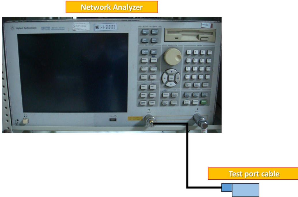
Figure 1. The schematic diagram for measuring VSWR
