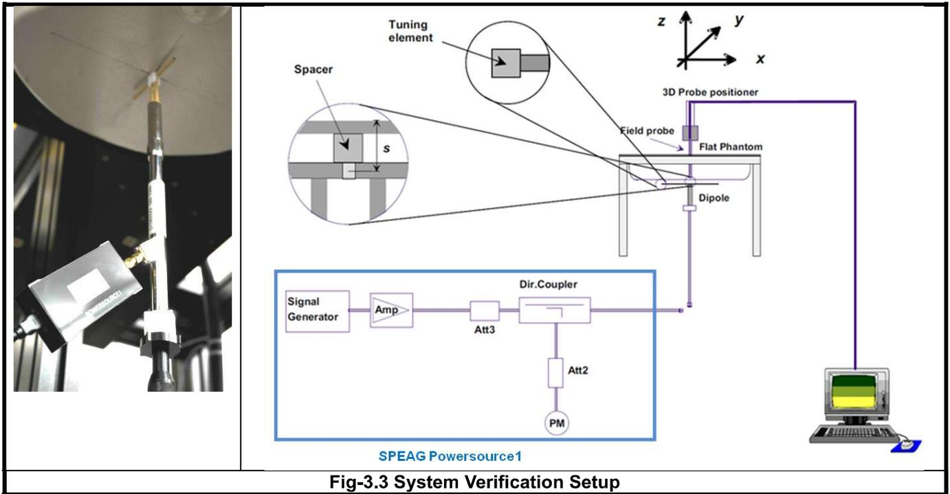
**Fig-3.3 System Verification Setup**
