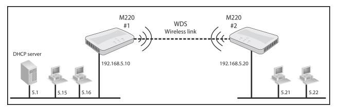
This example assumes that both M220s have their IP addresses set and are connected to their respective networks as shown in the diagram.
