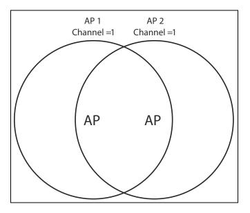
The solution to this problem is to set the two networks to different channels with as great a separation as possible in their operating frequencies. This reduces crosstalk and enables wireless clients connected to each M220 to transmit at the same time.
