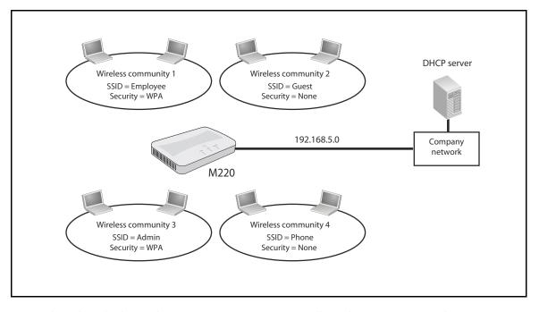
Even though multiple wireless communities are in use, all wireless users are on the same network (192.168.5.0). This means that all wireless users can reach resources on the corporate network. However, communication between wireless users may or may not be possible, depending on the configuration settings defined for each wireless community.
