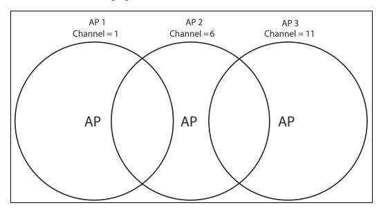
Alternatively, you can stagger APs to reduce overlap and increase channel separation, as shown in the following figure:
