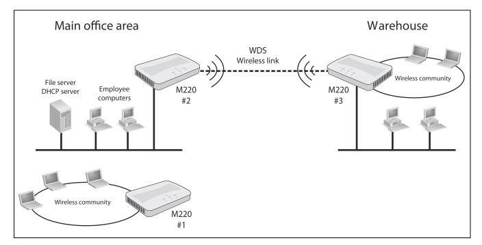
WDS links provide an effective solution for extending network coverage in situations where it is impractical or expensive to run cabling. Each M220 can create up to four WDS links.
