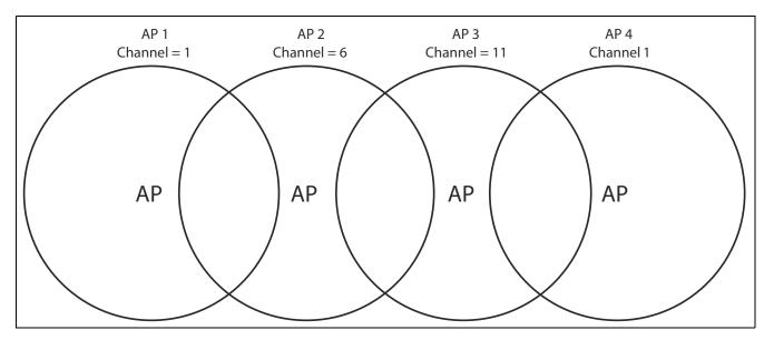
This strategy can be expanded to cover an even larger area using three channels, as shown in the following figure:
