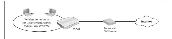
With its wireless community feature, the M220 can be configured to provide up to eight separate wireless networks (all on the same wireless channel), each with its own configuration settings for security, VLAN support, and more.
