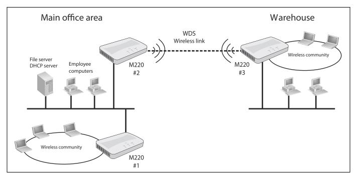
In the following scenario, three M220s provide distinct employee groups access to the Internet through a router on the network. The M220s are joined in a cluster, which enables them to share a single configuration and to be administered as a single unit. Channel planning may be implemented on the cluster to reduce interference and optimize wireless bandwidth usage.
