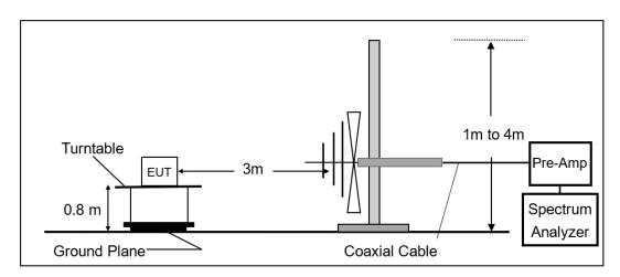
Radiated Emission Test Set-Up, Frequency Above 1GHz.
