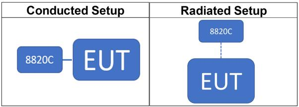
Note: Radio Communication Analyzer is placed in remote side for radiated test.
