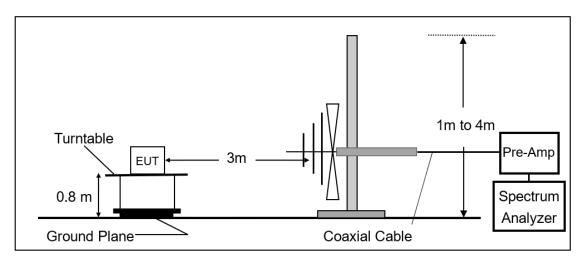
Radiated Emission Test Set-Up, Frequency Above 1GHz.
