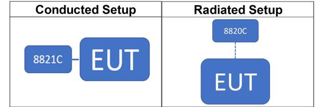
Note: Radio Communication Analyzer is placed in remote side for radiated test.
