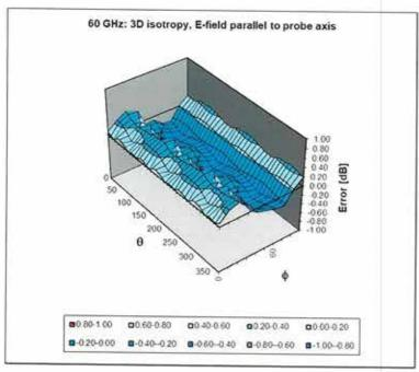
Probe isotropy for  $E_{tot}$ : probe rotated  $\phi$  = 0° to 360°, tilted from field propagation direction  $\overline{k}$  Parallel to the field propagation ( $\psi$  =0° - 90°) at 30 GHz: deviation within  $\pm$  0.36 dB Parallel to the field propagation ( $\psi$  =0° - 90°) at 60 GHz: deviation within  $\pm$  0.37 dB
