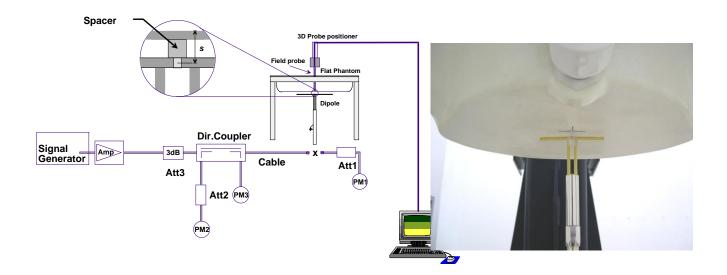
Fig 8.3.1 System Performance Check Setup
