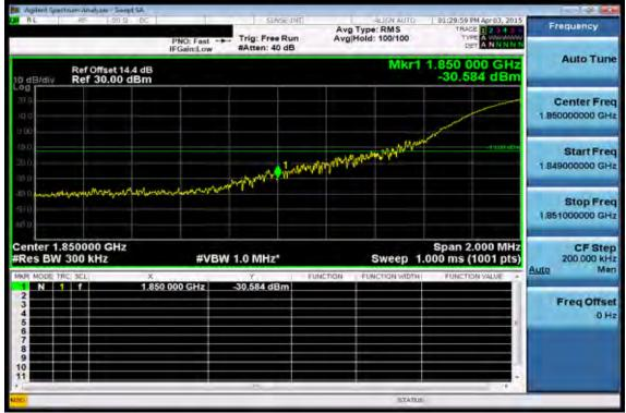
Band edge emission at antenna terminals -20MHz BW LTE-Band 25 (QPSK RB Number: 1 Offset: 99) Channel Highest
