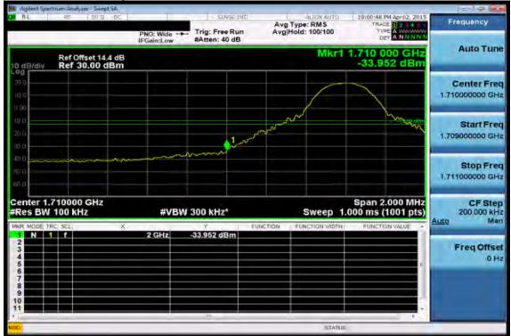
Band edge emission at antenna terminals -10MHz BW LTE-Band 4 (**QPSK RB Number: 1 Offset: 49**) Channel Highest
