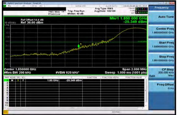
Band edge emission at antenna terminals –15MHz BW LTE-Band 2 (QPSK RB Number: 1 Offset: 74) Channel Highest
