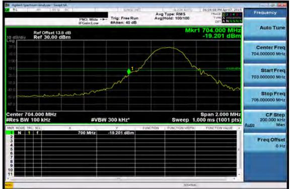
Band edge emission at antenna terminals –5MHz BW LTE-Band 17 (QPSK RB Number: 1 Offset: 24) Channel Highest
