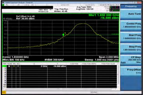
Band edge emission at antenna terminals -5MHz BW LTE-Band 25 (QPSK RB Number: 1 Offset: 24) Channel Highest
