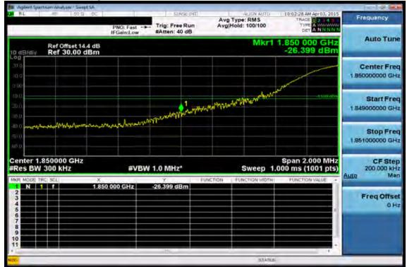
Band edge emission at antenna terminals -20MHz BW LTE-Band 2 (QPSK RB Number: 1 Offset: 99) Channel Highest
