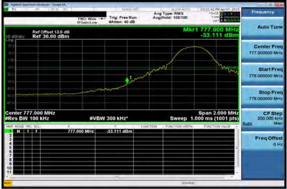
Band edge emission at antenna terminals -10MHz BW LTE-Band 13 (QPSK RB Number: 1 Offset: 49) Channel Highest
