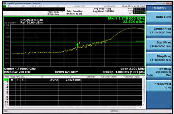
Band edge emission at antenna terminals –15MHz BW LTE-Band 4 (QPSK RB Number: 1 Offset: 74) Channel Highest
