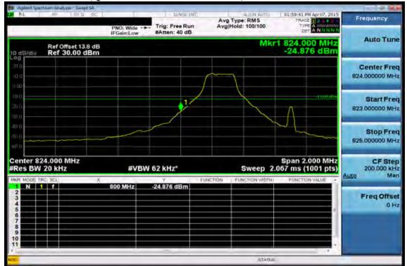
Band edge emission at antenna terminals –1.4MHz BW LTE-Band 5 (QPSK RB Number: 1 Offset: 5) Channel Highest
