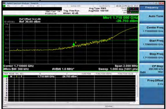
Band edge emission at antenna terminals –20MHz BW LTE-Band 4 (QPSK RB Number: 1 Offset: 99) Channel Highest
