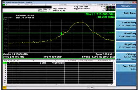
Band edge emission at antenna terminals -5MHz BW LTE-Band 4 (QPSK RB Number: 1 Offset: 24) Channel Highest
