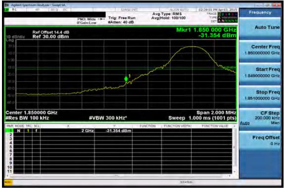
Band edge emission at antenna terminals -10MHz BW LTE-Band 25 (QPSK RB Number: 1 Offset: 49) Channel Highest
