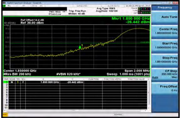
Band edge emission at antenna terminals -15MHz BW LTE-Band 25 (QPSK RB Number: 1 Offset: 74) Channel Highest
