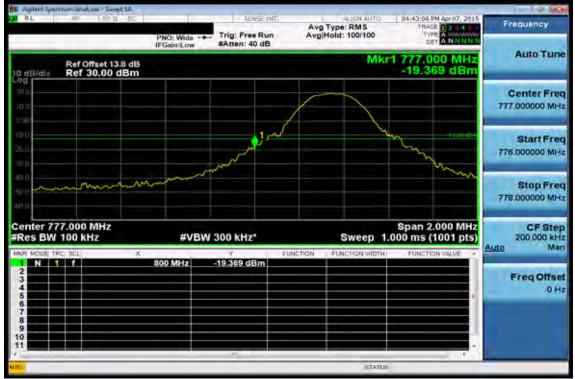
Band edge emission at antenna terminals -5MHz BW LTE-Band 13 (QPSK RB Number: 1 Offset: 24) Channel Highest
