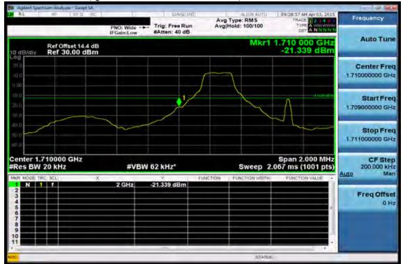
Band edge emission at antenna terminals -1.4MHz BW LTE-Band 4 (QPSK RB Number: 1 Offset: 5) Channel Highest
