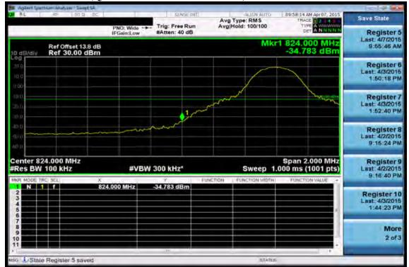
Band edge emission at antenna terminals –10MHz BW LTE-Band 5 (QPSK RB Number: 1 Offset: 49) Channel Highest
