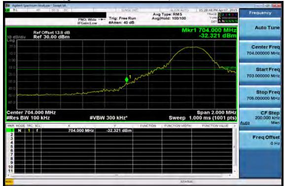
Band edge emission at antenna terminals -10MHz BW LTE-Band 17 (QPSK RB Number: 1 Offset: 49) Channel Highest
