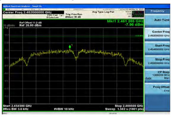
802.11g **Power Spectral Density Test Plot (CH-Low)**
