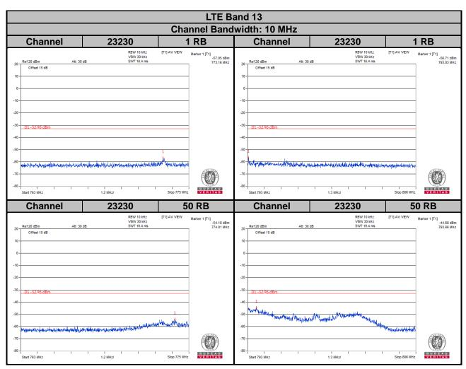
For the 763 - 775 MHz and 793 - 805 MHz band, the FCC limit is 65+10log(P[watt]) in a 6.25 kHz bandwidth. Since it was not possible to set the resolution bandwidth to 6.25 kHz with the available equipment, a bandwidth of 10 kHz was used instead to show compliance. By using a 10 kHz bandwidth on the spectrum analyzer.
