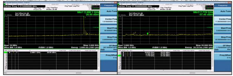
3GHz~20GHz Band41 10MHz QPSK 1 0 Low CH39700 30MHz~3GHz\_Band41\_10MHz\_QPSK\_1\_0\_High CH41540
