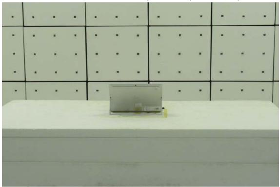
Radiated Emission Set up Photos (Below 1GHz) (E2 Plan)
