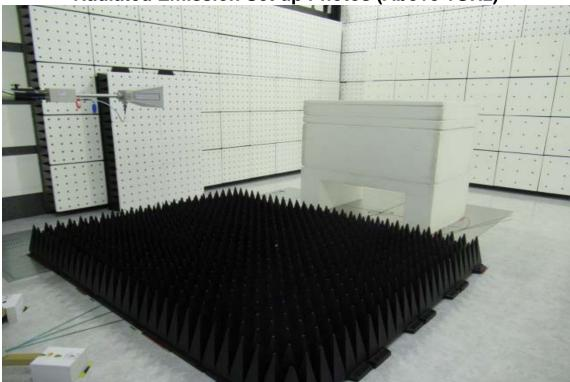
Radiated Emission Set up Photos (Front View)
