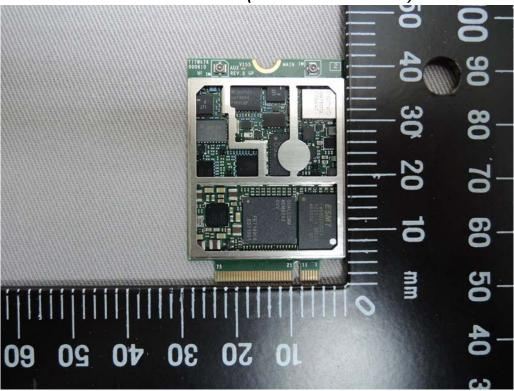
WLAN / BT Module - 1 (Model No.: 8265D2W)
