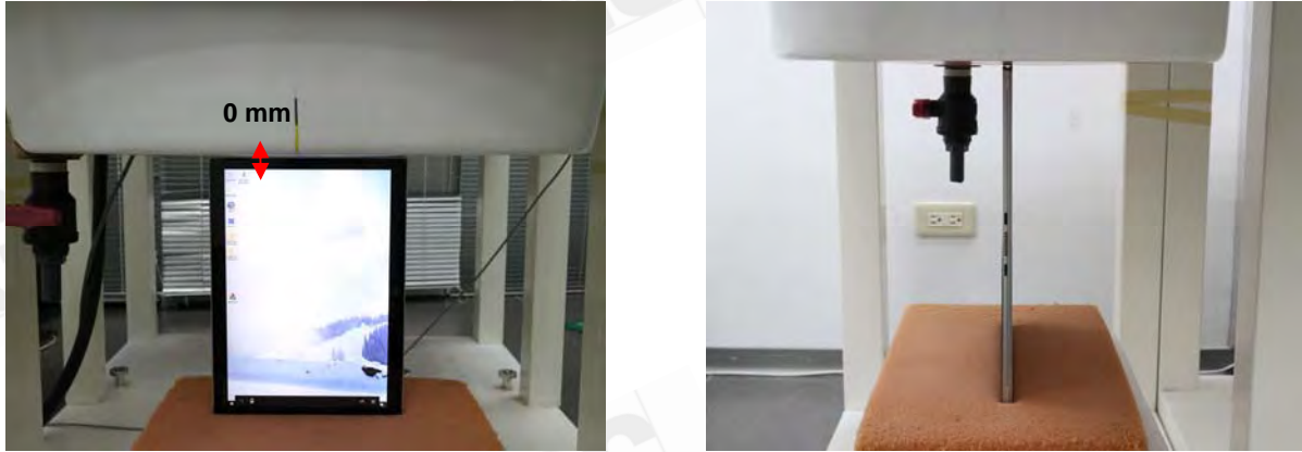
Fig.9 EUT Right side to flat phantom
