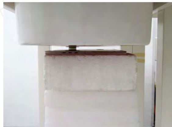
Fig.4 EUT Back side (14mm) to flat phantom
