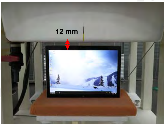
Fig.7 EUT Top side (12mm) to flat phantom
