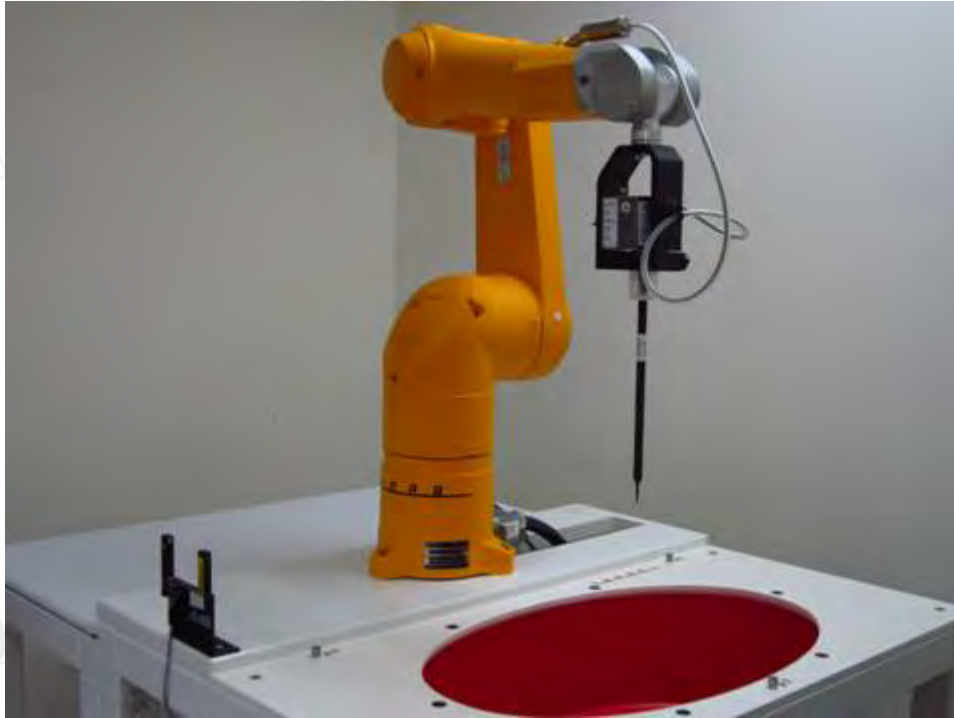
Fig.1 Photograph of the SAR measurement system
