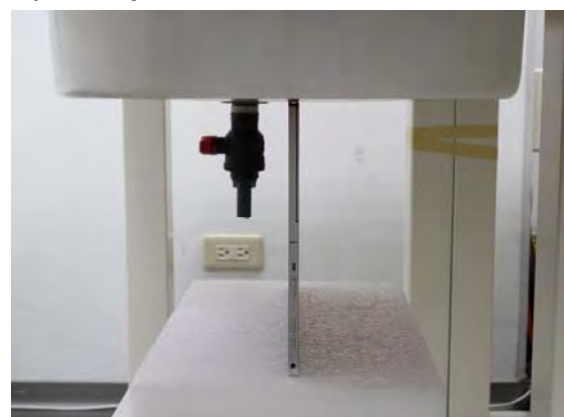
Fig.5 EUT Bottom side to flat phantom
