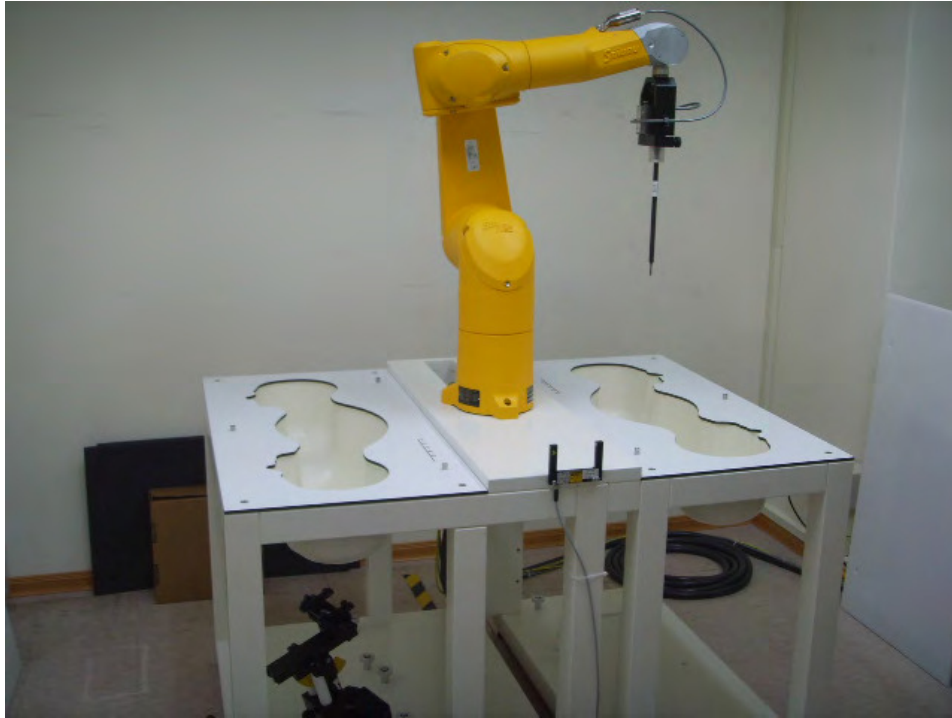
Fig.1 Photograph of the SAR measurement system
