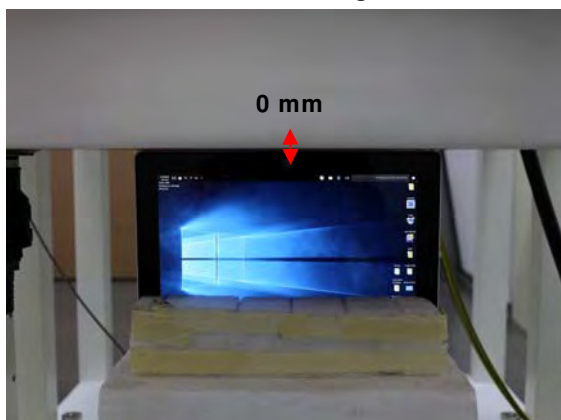
Fig.5 EUT Bottom side to flat phantom
