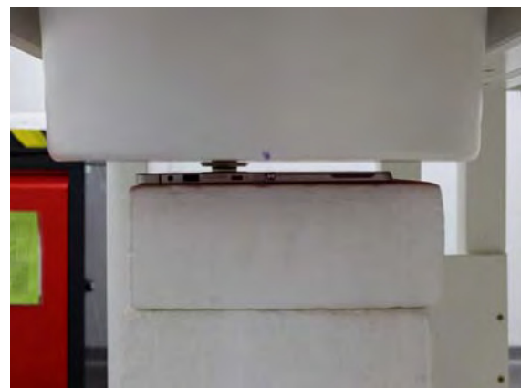
Fig.4 EUT Back side (10mm) to flat phantom
