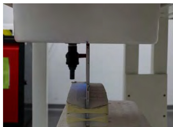
Fig.8 EUT Left side to flat phantom
