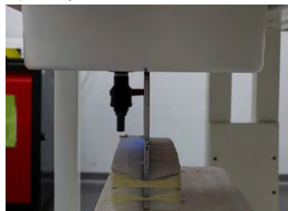
Fig.5 EUT Bottom side to flat phantom
