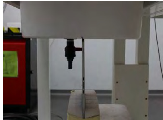
Fig.9 EUT Right side to flat phantom
