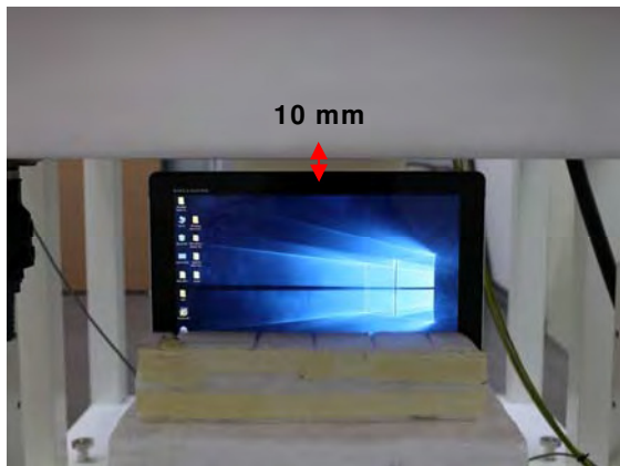
Fig.7 EUT Top side (10mm) to flat phantom
