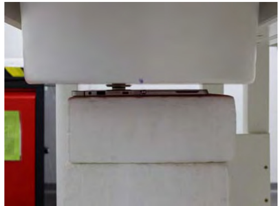
Fig.4 EUT Back side (10mm) to flat phantom
