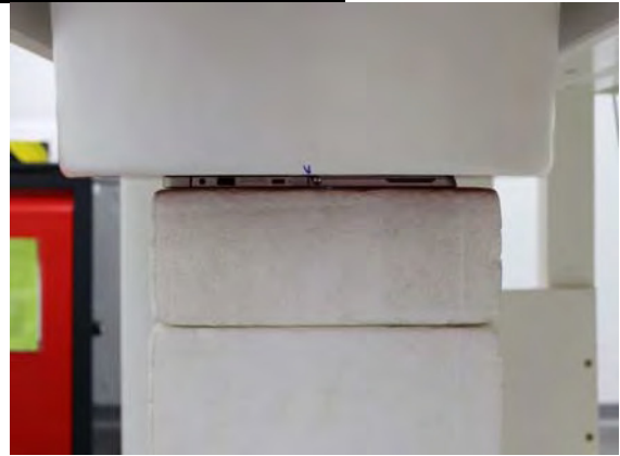
Fig.3 EUT Back side to flat phantom
