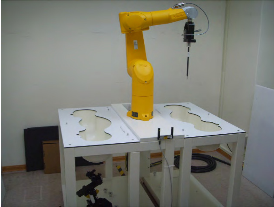
Fig.1 Photograph of the SAR measurement system
