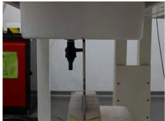
Fig.5 EUT Right side to flat phantom
