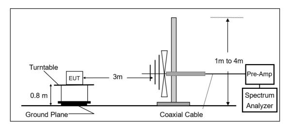
Radiated Emission Test Set-Up, Frequency Above 1GHz.
