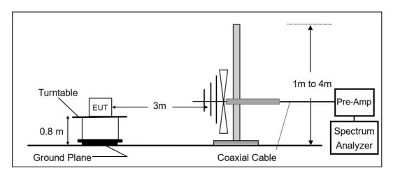
Radiated Emission Test Set-Up, Frequency Above 1GHz.
