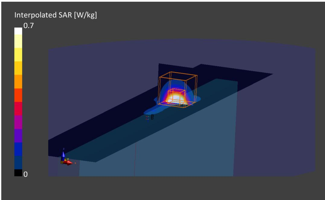
**26. System Check Body Liquid 750MHz – 2024-01-19**
