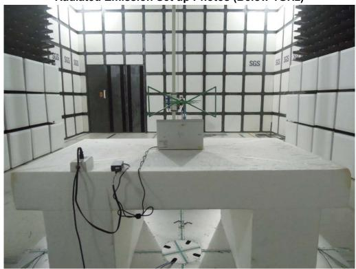
Radiated Emission Set up Photos (Above 1GHz)
