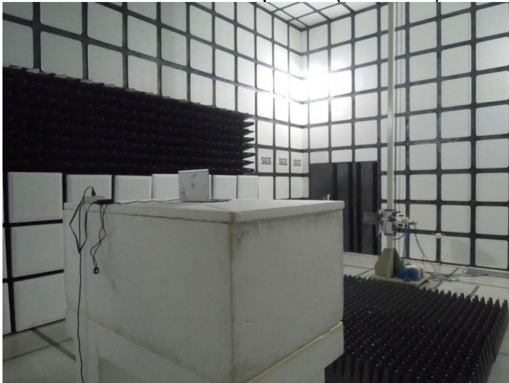
Radiated Emission Set up Photos (Above 1GHz)
