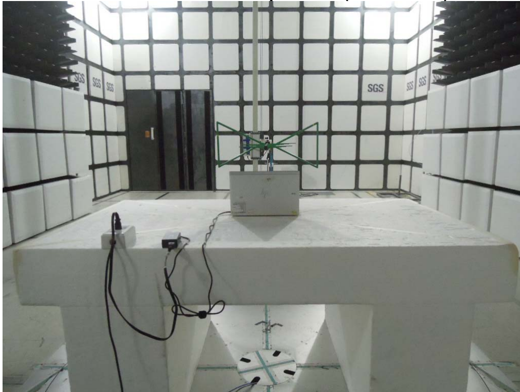
Radiated Emission Set up Photos (Above 1GHz)
