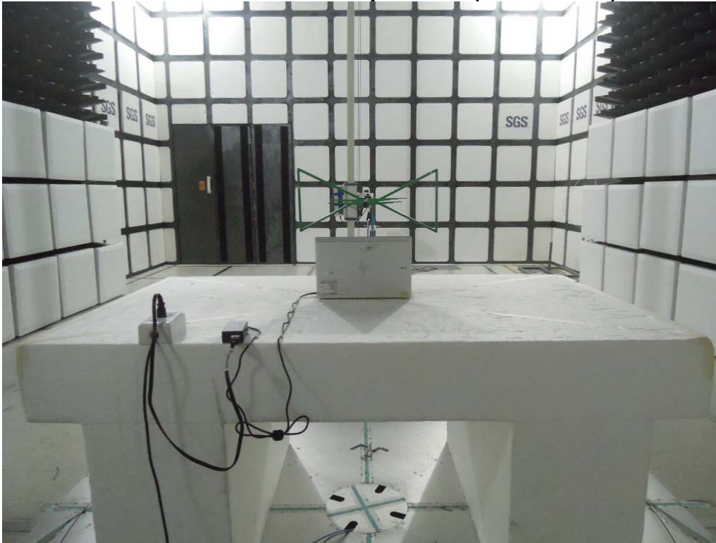
Radiated Emission Set up Photos (Above 1GHz)
