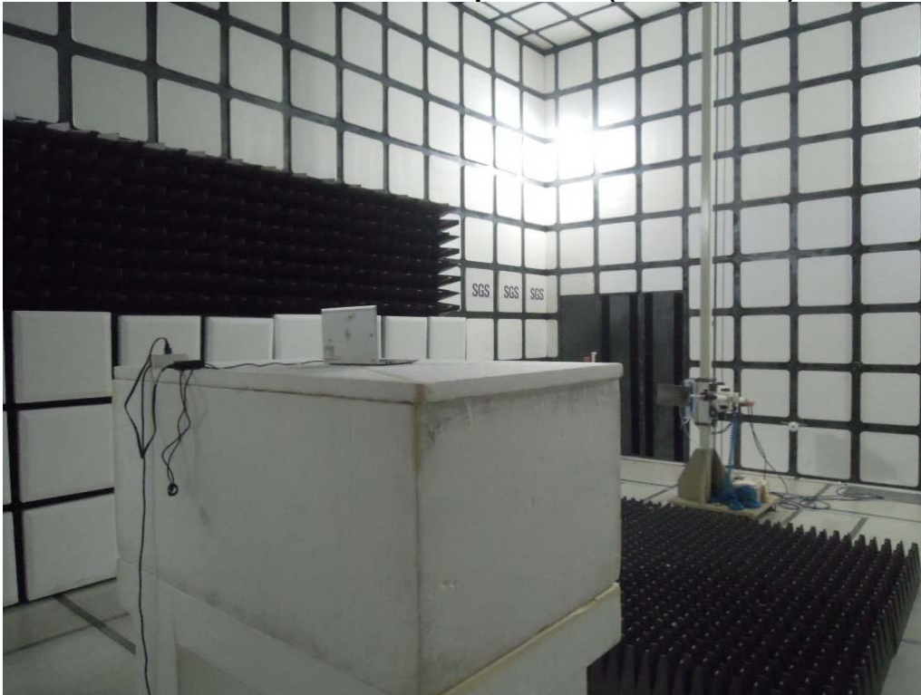
Radiated Emission Set up Photos (Above 1GHz)
