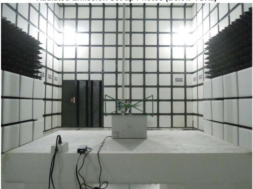
Radiated Emission Set up Photos (Above 1GHz)
