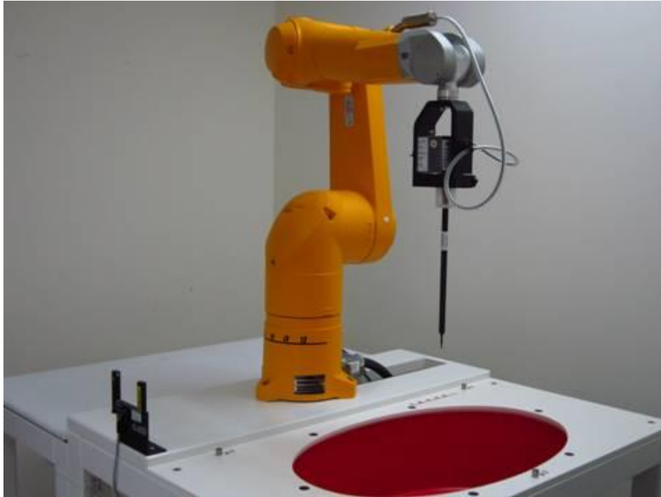
Fig.1 Photograph of the SAR measurement system
