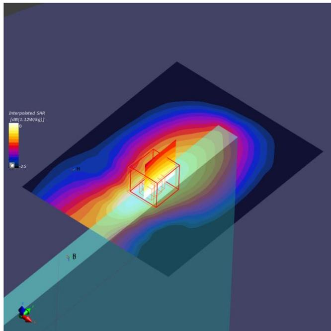
**9. LTE Band 25, QPSK - 20MHz, CH26365 , Main Antenna – Top Edge**
