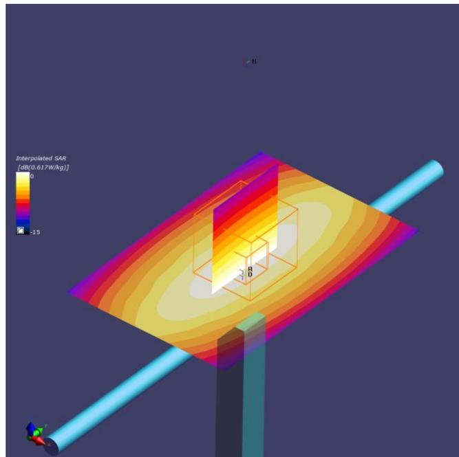
**16. System Check Body Liquid 750MHz – 2020-03-31**
