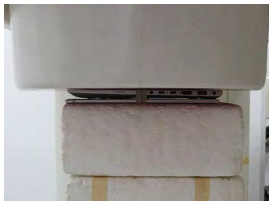
Fig.3 EUT Back side to flat phantom
