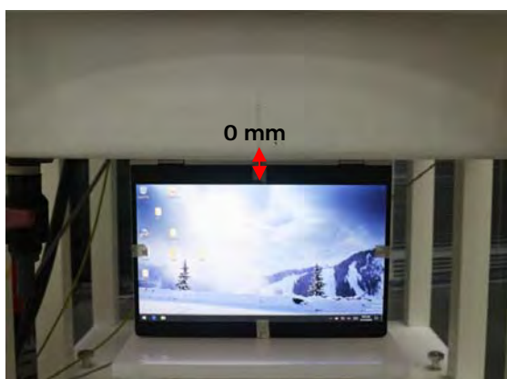
Fig.5 EUT Bottom side to flat phantom
