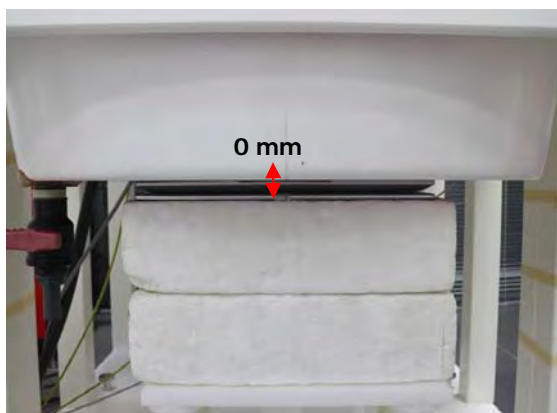
Fig.3 EUT Back side to flat phantom
