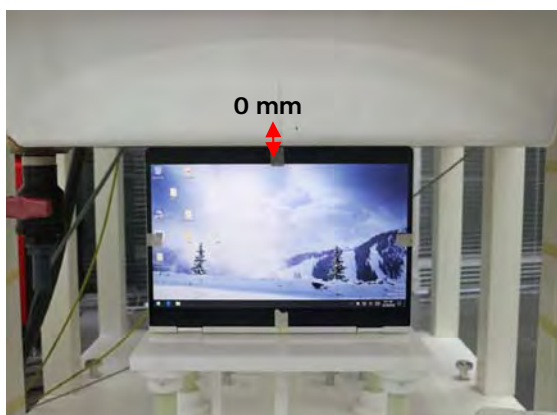
Fig.4 EUT Top side to flat phantom
