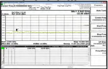
30MHz~3GHz Band26 Part90s 5MHz QPSK 1 0 MidCH26740-819
