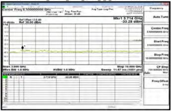
30MHz~3GHz Band12 5MHz QPSK 1 0 MidCH23095-707.5
