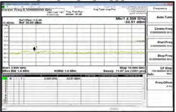
30MHz~3GHz Band26 Part90s 3MHz QPSK 1 0 MidCH26740-819
