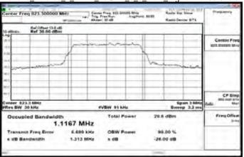
Band26 Part90s 3MHz QPSK 15 0 Main LowCH26705-815.5
